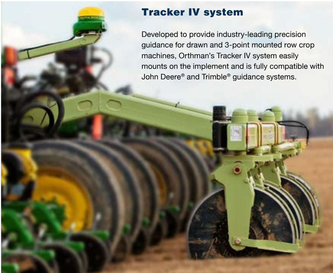
Available with 2, 3, 4 or 6 ground-engaging steering blades, the Tracker IV design features a single hydraulic cylinder that pivots all the blades simultaneously for consistent implement-tracking correction. The Tracker IV is available with 20" to 40" row spacing to fit your operation.
