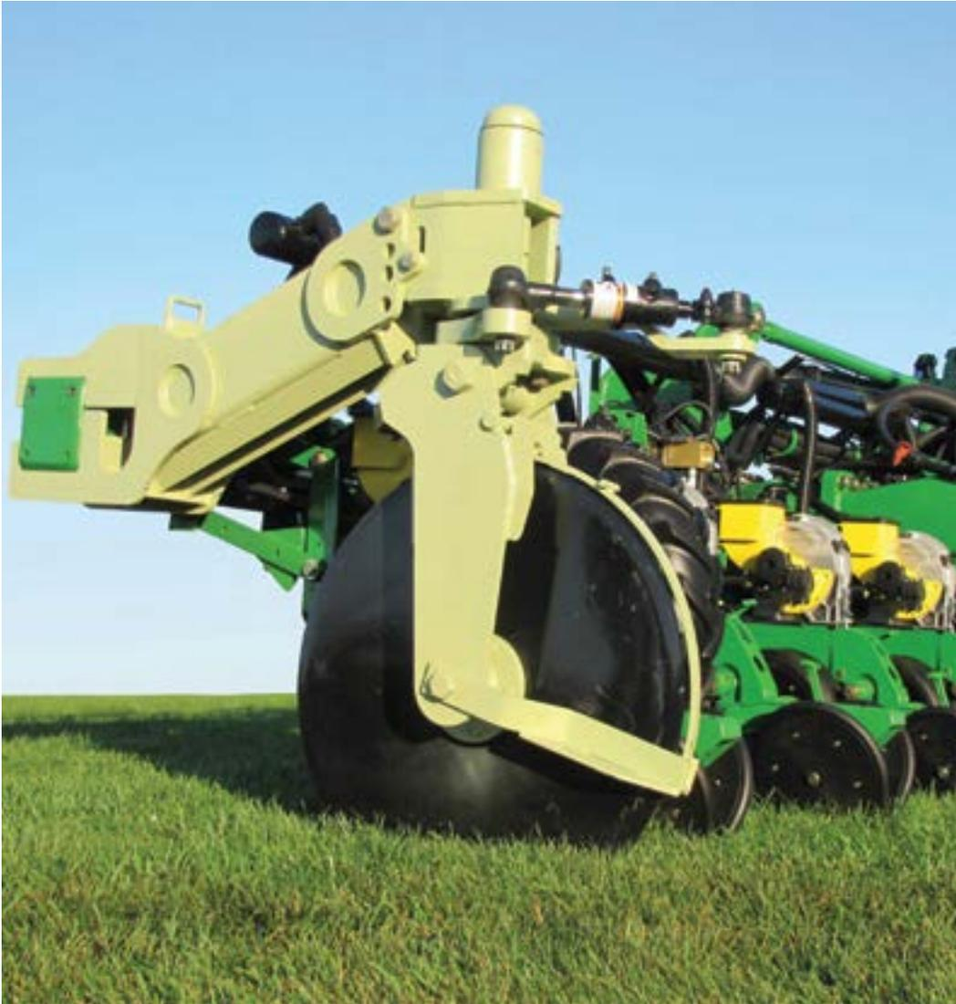
Based on the same operating principles as the Tracker IV, the Shadow Tracker includes a single cylinder and blade that can be mounted in combinations of up to 4-blade systems depending on the size of the implement and field terrain.
