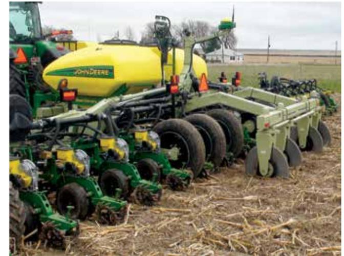
The Tracker IV™ system uses a 5x7x3/8" crosstube with bolt-on mounting arms attaching it to the existing toolbar. It is available in 2, 3, 4 and 6 blade models, based on implement type and size. Drawn implements have the ability to travel laterally more than hitched implements. Sway bars should be removed when using hitched implements to allow the Tracker to adequately correct implement position.
